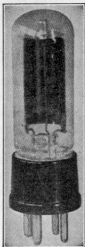
FIG. 171.—Typical photoelectric tube.
